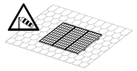
When installing on a roof, ensure that the roof construction is suitable. In addition, any roof penetration required to mount the module must be properly sealed to prevent leaks.
