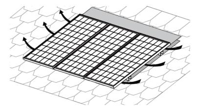
Provide adequate ventilation under a module for cooling. 50 mm minimum between the module and the mounting surface.
