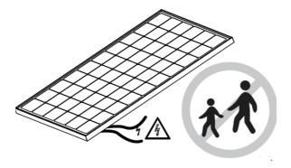
Revision 22 Jan 22 Page 15 of 36 Completely cover the module with an opaque material during installation to keep electricity from being generated. Do not touch the ends of live wires. Do not wear metallic rings, watchbands, ear, nose lip rings or other metallic devices while installing or troubleshooting photovoltaic systems
